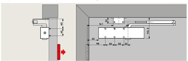
With parallel arm application, the backcheck comes in later at between 85° and 90°, depending on the door thickness and projection of the hinge used; the delayed action, on the other hand, releases the door at an earlier point in its closing sweep.
