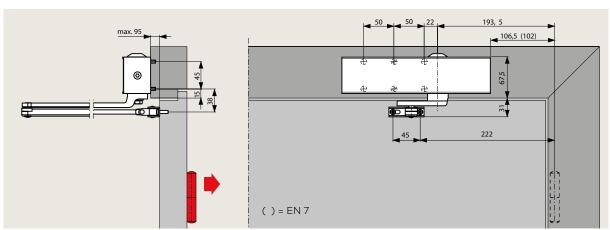
With transom-fixed closers, the backcheck only responds at between 85° and 90° depending on the depth of reveal and type of door hinge involved; the delayed action, on the other hand, releases the door at an earlier point in its closing sweep.
