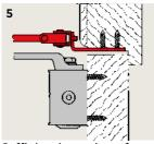
Soffit bracket and arm for standard installation with shaped architrave
